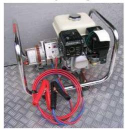
This larger model is best suited for larger charging requirements, such as the marine industry, backup for solar powered sites, motor-homes, earthmoving contractors, emergency services, mobile mechanics, communication repeaters, arrow boards, council machinery etc. Designed for the harsh environments of Australia, so no digital electronic components are installed on this model.
